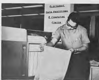
THE PRINTER can be loaded with paper in a matter of seconds. Since skipping between printed lines is up to sixty times as fast as printing, faster document output can be obtained than just from printing speed alone. E IMPRESOR por worde yená cu papel den poco seconde. Como un cambio pa otro linea ta como sesenta bez mas rapido cu drukmento mes, ta mas liber pa completá un documento cu si mester depende ariba velocidad di drukmento sol.
